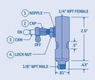
To set or change rate of flow, push cam (3) to horizontal position. Loosen lock nut (4). Turn cap (2) counter clockwise until oil is feeding properly. Lock setting with lock nut (4).
