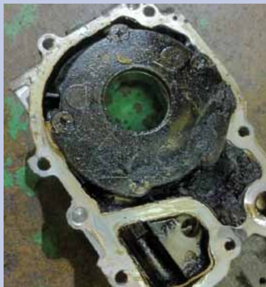
ABOVE: The dangerous affects of oil degradation on internal components.
